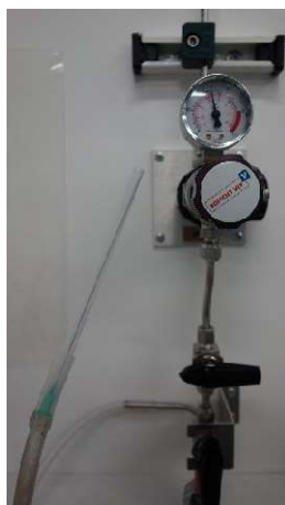
Figure 2-1: Needle used to degas the reactors with Ar.
